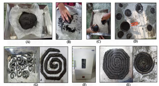
(A) Composition of Mixture, (B) Added boiled water, (C) Thick and consistent paste formed, (D) Paste was rolled into a thin ribbon, (E) Moist coil shape was formed, (F) Coil was left inside the oven, (G) Dried marigold based coil
