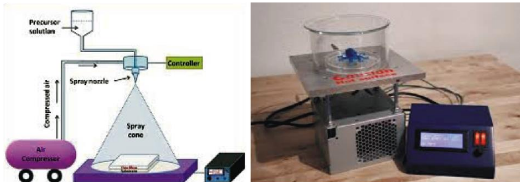
Figure 2: Spray pyrolysis setup including PID temperature controller, hot plate, and spray gun.
